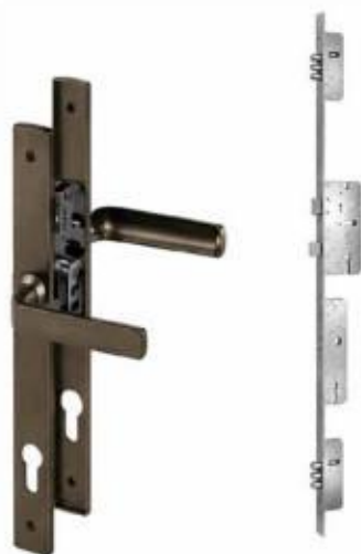
16 mm Faceplate Mechanical Multi-Point lock on Euro-groove (6 to 8 locking points) operated by European Style Trims .
